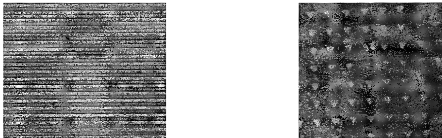
Figure 8. Deposited copper left 5 \mu\text{m} lines of polymer (2) right: 10 \mu\text{m} triangles of polymer (4)
